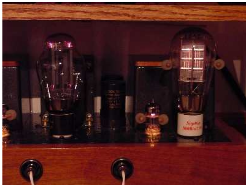
Sophia 274B Rectifier and the 2.5 Volt 300B (2A3) Meshplate
